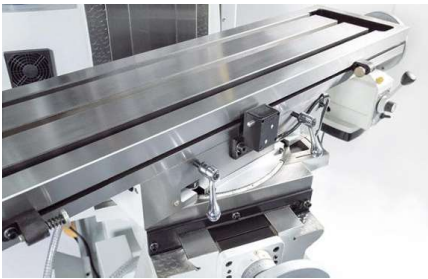
Cutter table swivels in X axis
