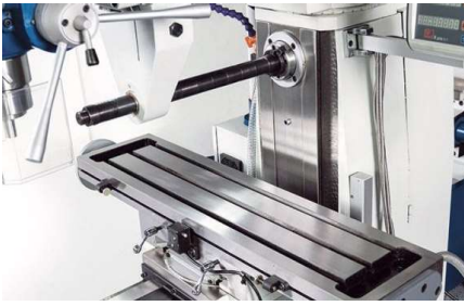
Solid top beam with outer arbor allows rigid mounting of long milling arbors
